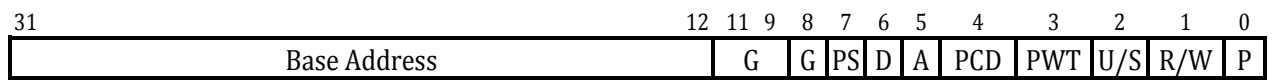
Fig. 4.7. Format of the pointer to the page table of the IA-32 architecture
