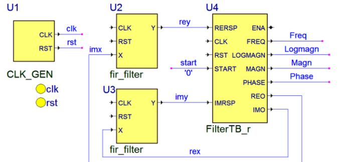
Fig. 3. Testbench for the filter response computation
