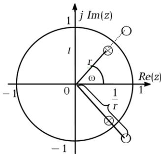
Fig. 1. Pole-zero chart of the all-pass filter
