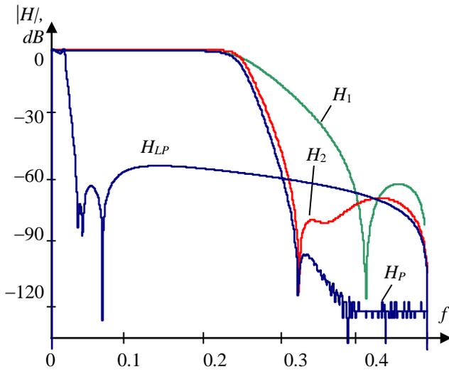
Fig. 5. Frequency response characteristics of the synthesized filters
