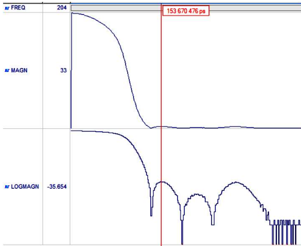
Fig. 18. The magnitude-frequency response and the logarithmic frequency response of the filter in Fig. 17
